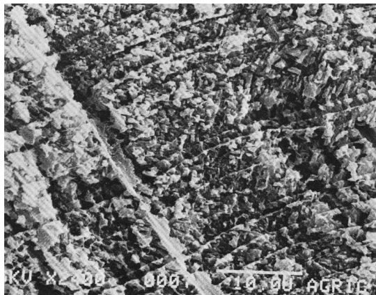
Figure 51. Scanning electron micrograph of the fixed, etched, and critical point dried shell of the benthonic foraminifer, Heterostegina depressa , showing the lamellae separated by organic matrix layers. Note that the shapes of individual crystals are very difficult to identify (scale bar = 10 \mu\text{m} ). Reprinted with permission from ref 362. Copyright 1986 CRC Press.
